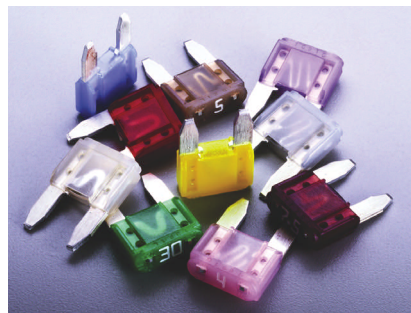
FIGURE 2. Automotive fuses, such as these in blade packages, undergo life tests that last 100 hr.
