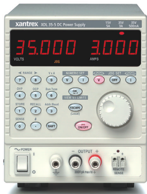
As quiet linear sources, remote-sensing power supplies from Xantrex exhibit less than 0.35-mV RMS voltage noise and less than 0.2-mA RMS current noise. Courtesy of Xantrex Technology.
